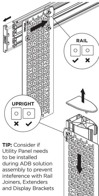
**TIP:** Consider if Utility Panel needs to be installed during ADB solution assembly to prevent interference with Rail Joiners, Extenders and Display Brackets
