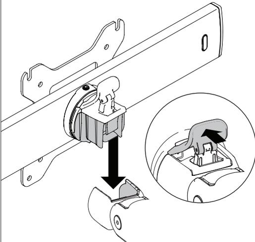
**Note:** Ensure the lever is unlocked when fitting.
