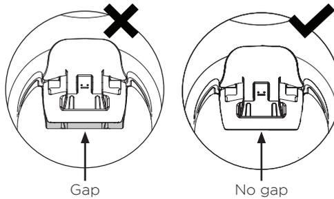
**2.3** Push the lever down to secure it to the arm assembly
