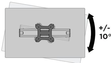
**3.3 (Optional)** Monitor rotation tension may be adjusted by tightening or loosening a small screw with the provided allen key.
