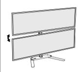
**8.2** To close small gap between displays +/-6mm (1/4"):
