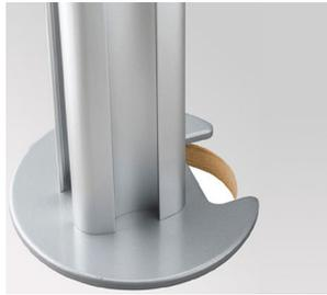
Utilises an existing grommet hole or can be used as bolt through fixing. The plate provides extra stability for heavy loads. Fits grommet holes 2.36"-3.15" in diameter.
